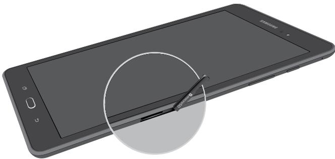
2. With the gold contacts facing down, carefully slide the memory card into the slot, pushing gently until it clicks into place.
